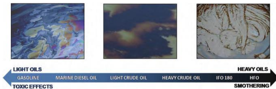
▲ Figure 2: Typical effects on marine organisms range across a spectrum from toxicity (especially for light oils and oil products) to smothering (intermediate and heavy fuel oils (IFO and HFO) and weathered residues).
